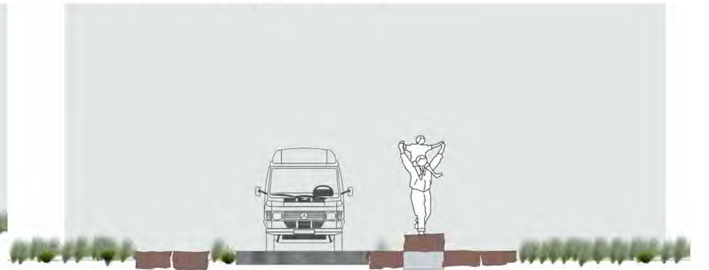
Extra wide shared paths allow for safe use and movement for multiple users including cycling, mobility scooters, jogging and pedestrians. The width also provides access to service and maintenance vehicles to ensure ease of site maintenance.
