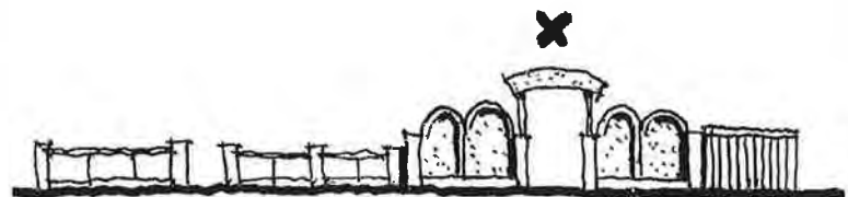
The fence designs on the right have greater solid to void ratios.
